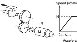
Speed (rotational) vs Time graph showing a linear increase from 0 to N over time t<sub>A</sub>.
