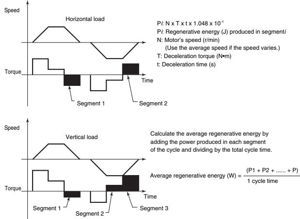
**Note:** 1. The speed is positive when the motor is rotating forward and the torque is positive when it is in the forward direction.
