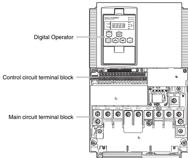
**Note:** This illustration shows the terminal block with the Terminal block front cover removed.
